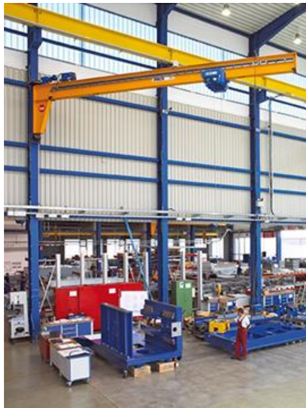
Figure 1: Jib-crane, wall mounted, ‘T’ version, using the I beam of the structure as mast 1 .
